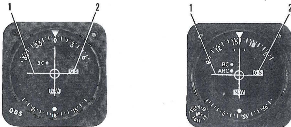
1. GLIDE SLOPE DEVIATION POINTER - Indicates deviation from normal glide slope.
